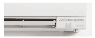
Our Pro-Heat™ wall-mounted models have the 3D i-see Sensor™. This infrared human sensing device scans the room and discovers the location of human heat signatures. The sensor also measures floor temperature in order to deliver conditioned air to those occupied areas that need it using double-vane airflow and motorized vertical vanes.
